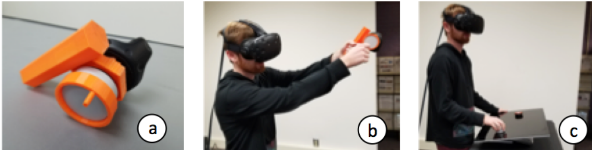
Figure 1. a and b) Rod and reel tangible combining a Vive tracker, Microsoft Surface Dial and 3D printed elements for a fishing simulation. c) Student operating VR interface with the Microsoft Dial on top of a multi-touch display.
