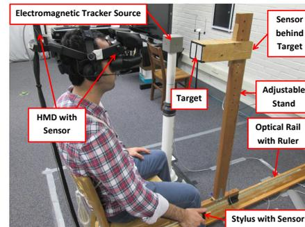
Figure 1: The near-field distance estimation apparatus.
