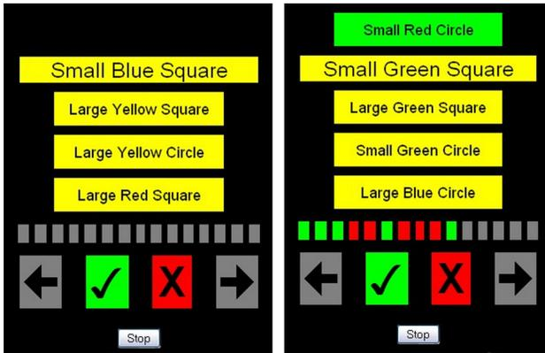
**Fig. 2** Visual display for handheld configuration using an abstracted task list. Left: the handheld GUI when the application starts. Right: the GUI after several items has been checked off. The most recently checked item is green because it passed inspection, and the progress bar is color coded according to the inspection results of all items checked so far.
