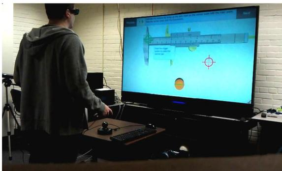
Figure 4: A user interacts with the virtual calipers using a two-handed 6 DOF controller
