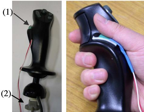
Fig. 3 Spatial mouse with attached FSR (1) and receiver (2).
