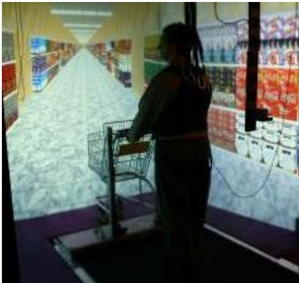
Figure 1. Subject walking through virtual grocery store while pushing on physical grocery cart instrumented with force transducers. The speed of the treadmill and movement through the store is proportional to the amount of force applied to the cart handle. Speed is limited to 1.2 m/s.
