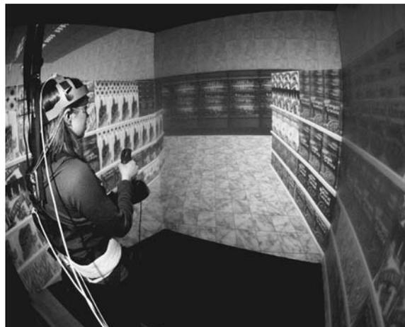
**FIG. 1.** The Balance NAVE Automatic Virtual Environment (BNAVE) includes a Neurotest force platform surrounded on three sides by back-projected screens displaying a virtual grocery store environment. The subject is supported by a harness, and is wearing a Polhemus Fastrak sensor on her head to measure head movements.
